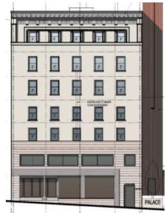
Windows in front facade below were restored to original – those at left were added to blank wall on side/ non-street elevation
