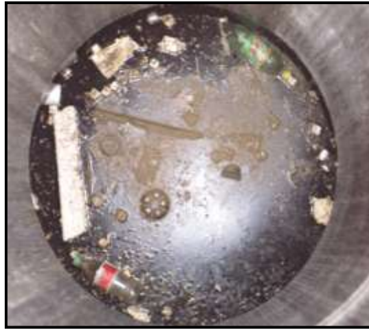
Floatable debris in the Aqua-Swirl®
