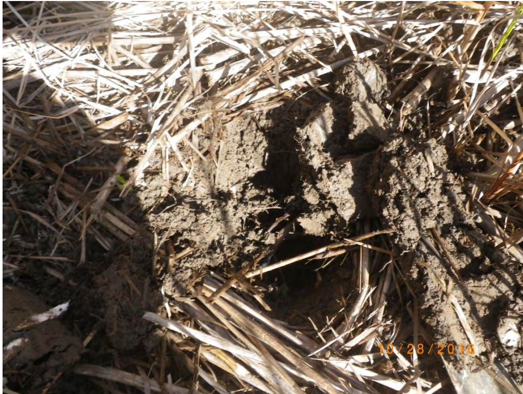
Photo 4 Hydric soil features in sample pit
