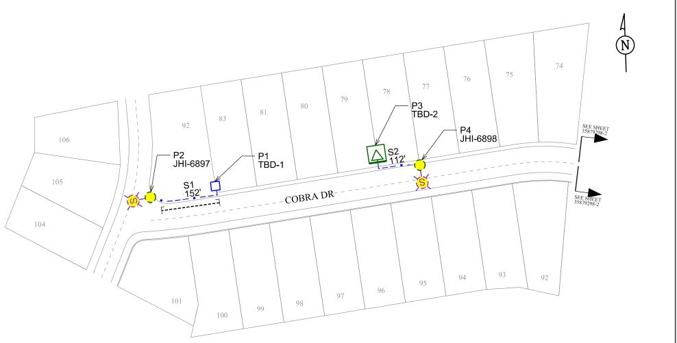
AMS TO INSTALL 2" CONDUIT AT 36" DEPTH FOR DUKE LIGHTING AT LOCATION S1.
