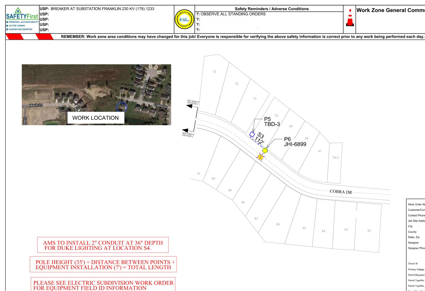
S INSTALL 50W LED ROADWAY ST LT ON 35' CL5 WOOD POLE W/ 18" BKT/MAST. SET POLE 3' BACK OF CURB AND ON PROPERTY LINE, UNLESS NOTED (W.C. \*ICAL) TOTAL-3
